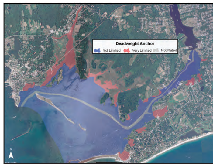
Fig. 5. A map of the mooring interpretation for deadweight anchors in Little Narragansett Bay based on the bottom type of soil material.
